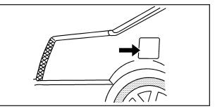
To open the fuel door, apply pressure in the center of the rear edge of the fuel door and it will pop open. To remove the fuel cap, turn it slowly counterclockwise. The fuel cap has a spring in it; if the cap is released too soon, it will spring back to the right.
